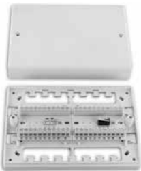
Surface-mounted screw-type distributor 20-pin model 7458-20 20-pin distributor in plastic, surface-mounted version with screw-type terminals. Serves as an interconnection point between flexible cabling in the door and the building wiring installation, or as a junction point where clearly arranged wiring branches out to several door systems. With cover contact for sabotage monitoring.
